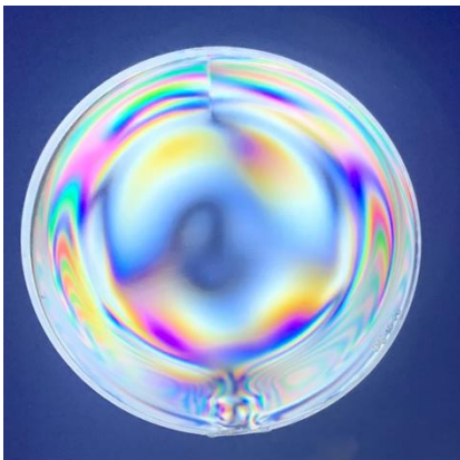
75mm Polymer Lens Commercial Molding
